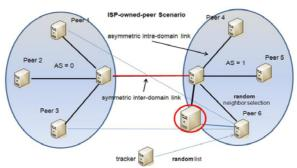
Fig. 4.1: Insertion of ISP-owned peer in pure BT.
